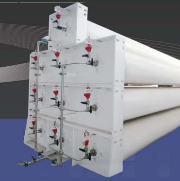
The storage vessels are mainly used for CNG charging stations, industrial factories & ships. Three vessels of 1,300 liters combined into one module are standard structure. In case of larger storage stations, several more modules can be installed. The specifications for vessel design, manufacture and inspection comply with the ASME standard of USA as well as the standard of Korea Gas Safety Corporation.
