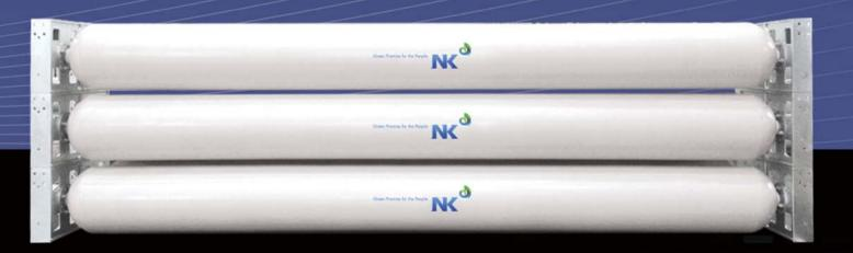
NK Group has delivered various Air Pressure Vessels to customers in order to obtain constant tension in the marine drilling riser. Air Pressure Vessel is connected to the Piston accumulators air-side in Marine riser tensioner system. This means that the riser tensioner unit acts like a hydro/pneumatic spring by using the compressed air from Air Pressure Vessel. These ultra high pressure vessels have also special demands from aerospace centers for rocket launching program.
